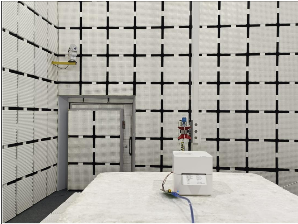
RADIATED EMISSION TEST (1GHz ~ 18GHz)
