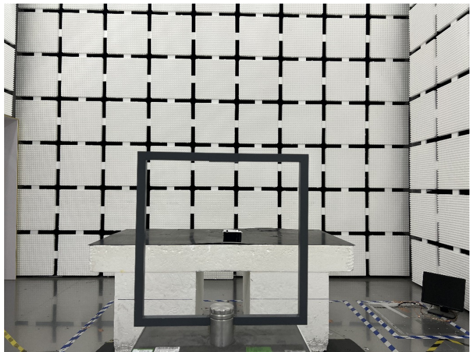
Radiation Emission Test Setup (Below 30MHz)
