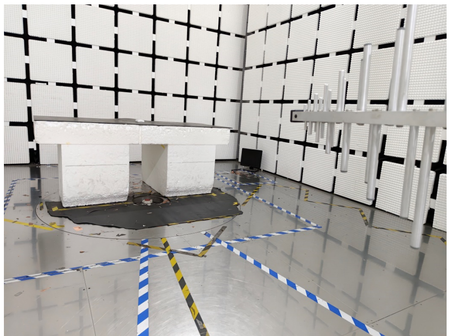
Radiation Emission Test Setup (30MHz to 1GHz)
