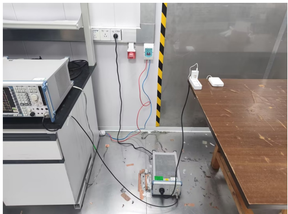
Conducted Emission Test Setup
