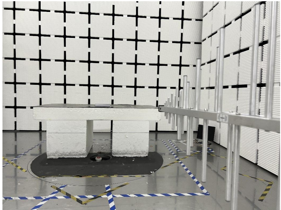
Radiation Emission Test Setup (30MHz to 1GHz)
