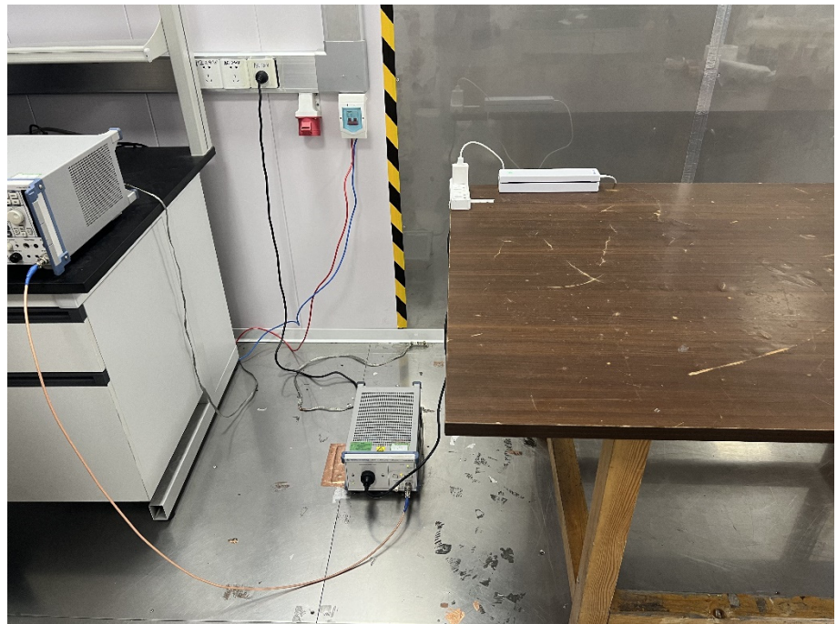
Conducted Emission Test Setup
