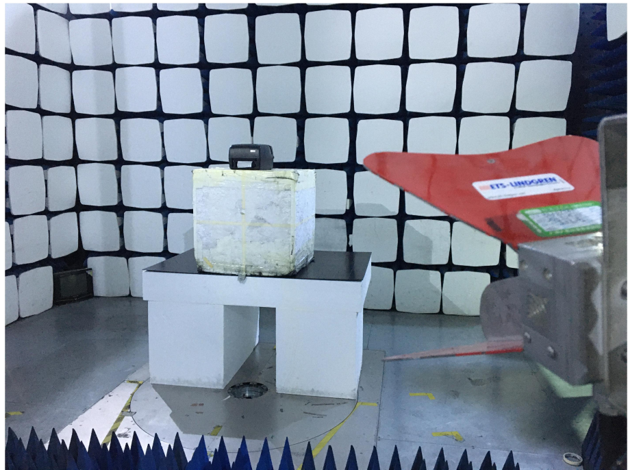
Radiation Emission Test Setup (1GHz to 18GHz)
