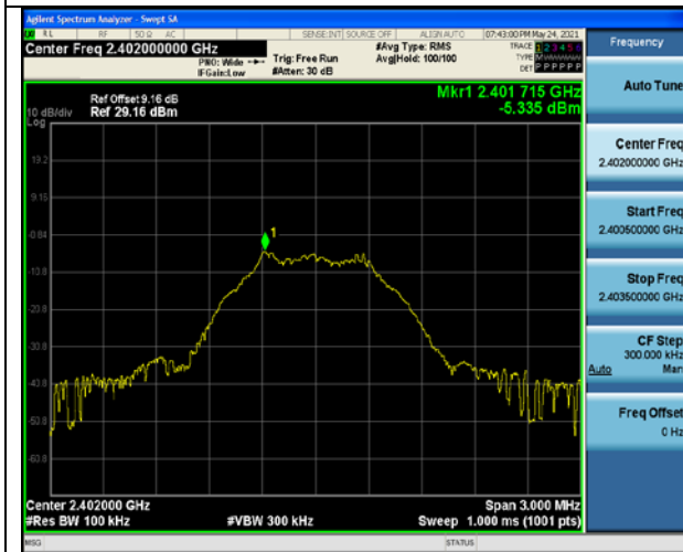
GFSK on Channel 00
