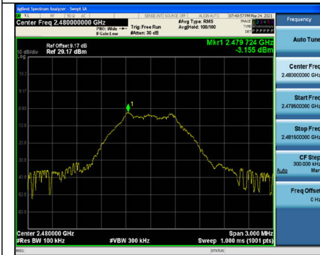
GFSK on Channel 39
