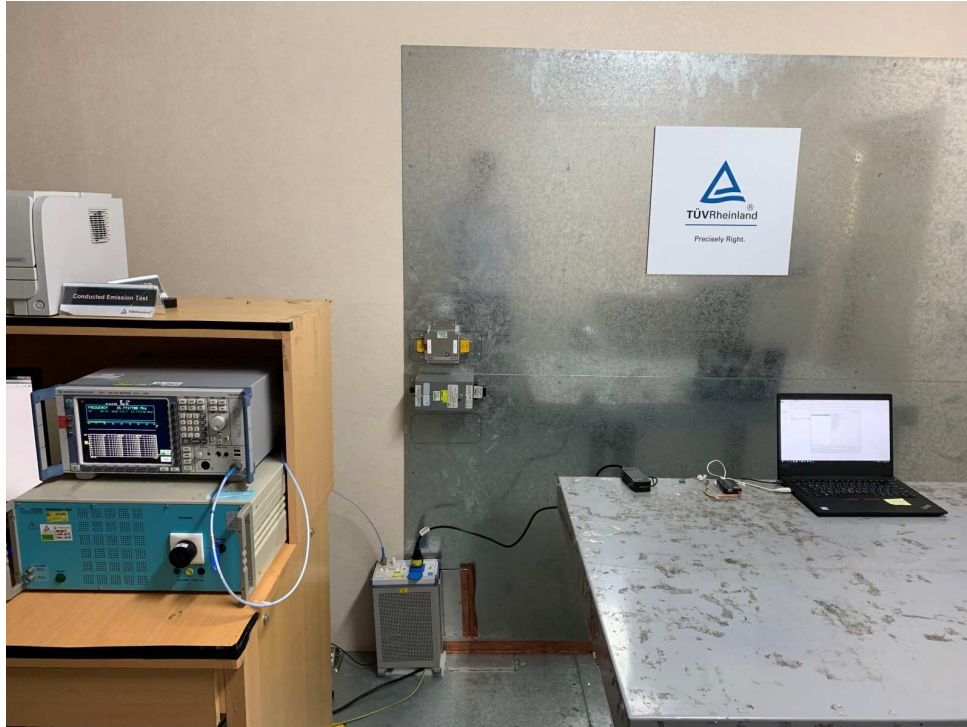
Photograph 9: Set-up for Mains Conducted testing (Front View)
