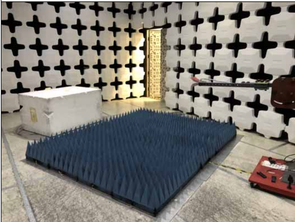
Test Setup for Radiated Emissions: Above 1GHz, Vertical Polarization
