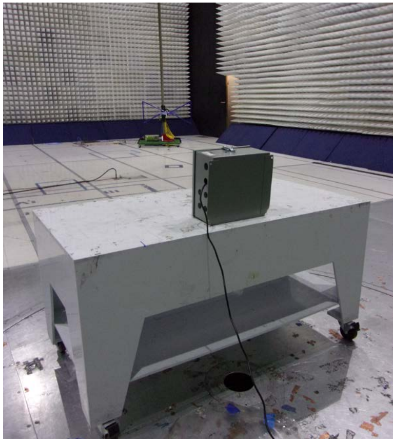
Electromagnetic Radiated Disturbance Setup Photograph
