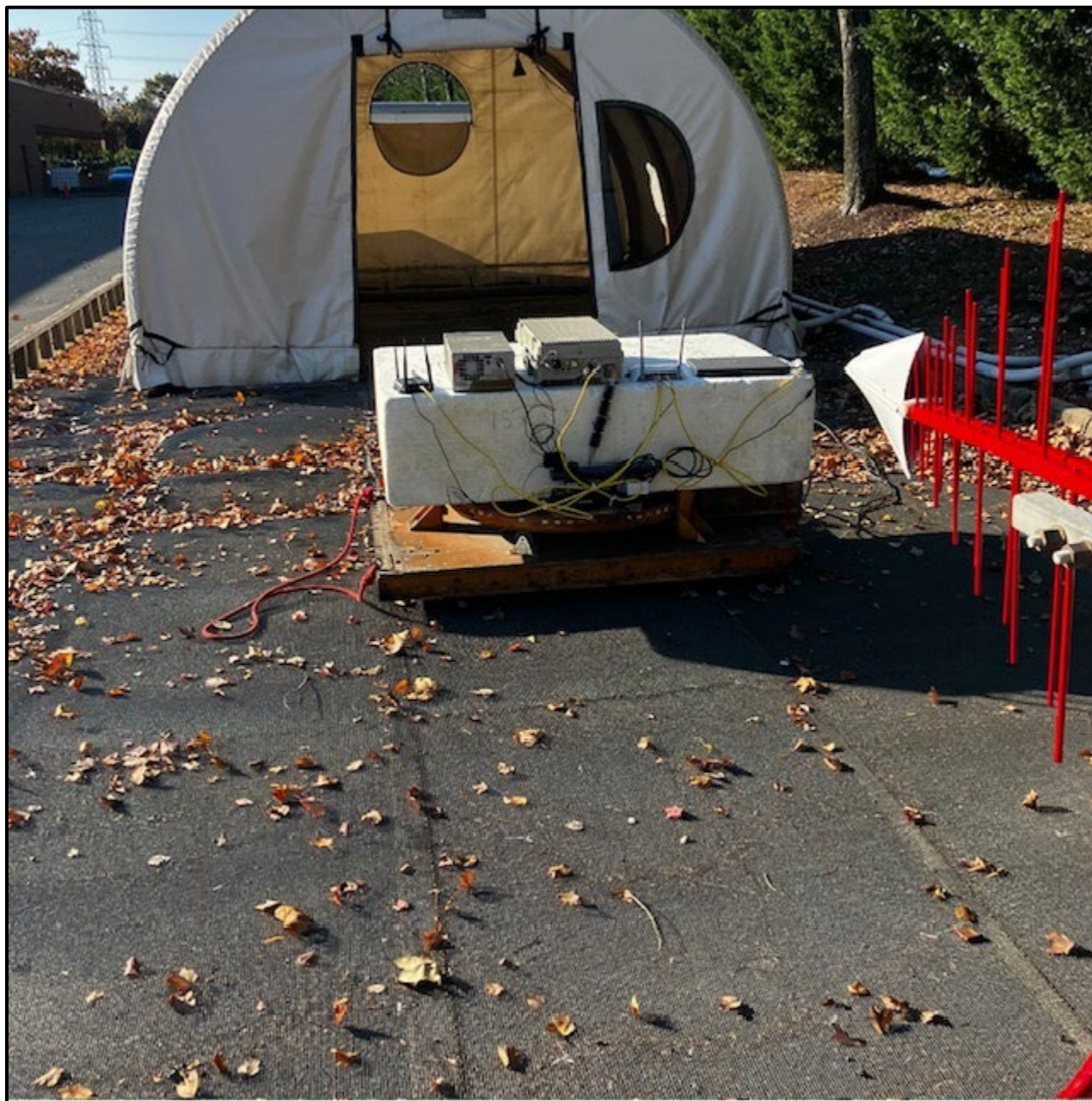
Photograph 2: Radiated Emissions – Back View (Below 1 GHz)
