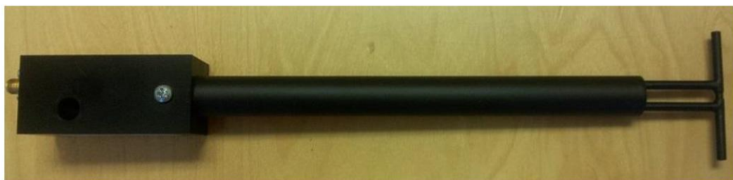
Figure 1 – MVG COMOSAR Validation Dipole
