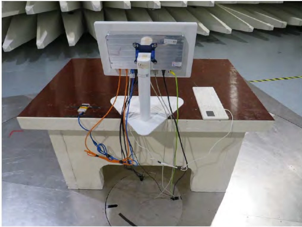
OR-PC® 21 Radiated Emission Test Setup 30 - 1000 MHz
