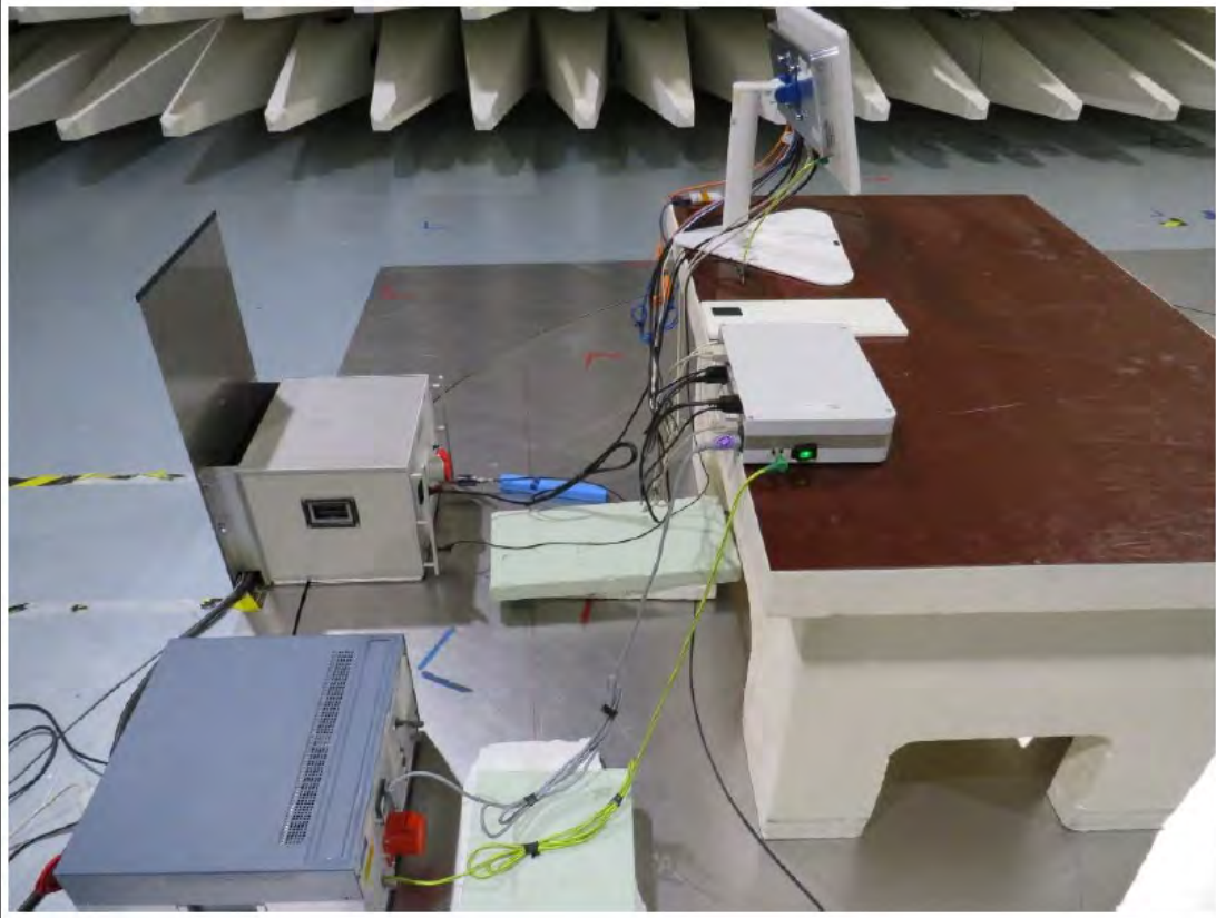
OR-PC® 21 Conducted Emission Test Setup
