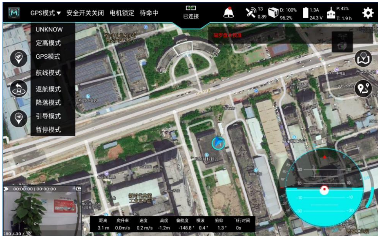
Figure 9 route mode drop-down box
