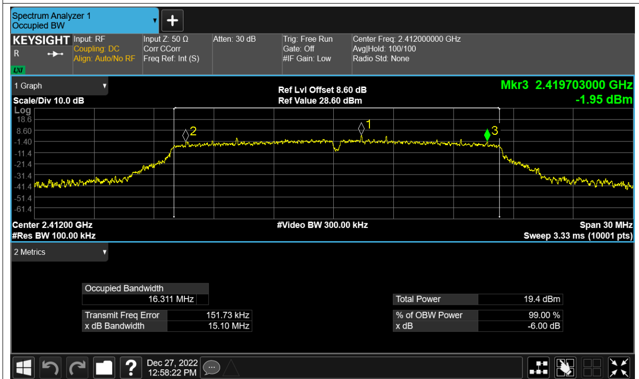
-6dB Bandwidth NVNT g 2437MHz Ant1
