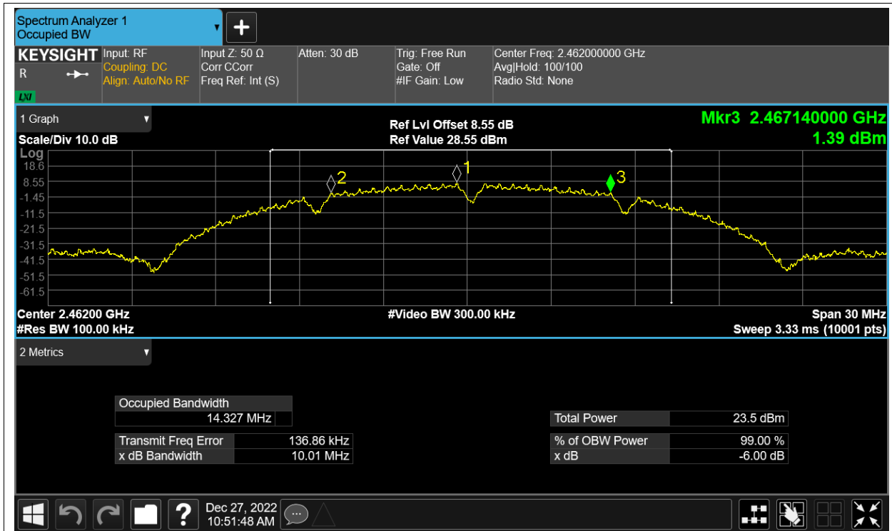
-6dB Bandwidth NVNT b 2437MHz Ant2
