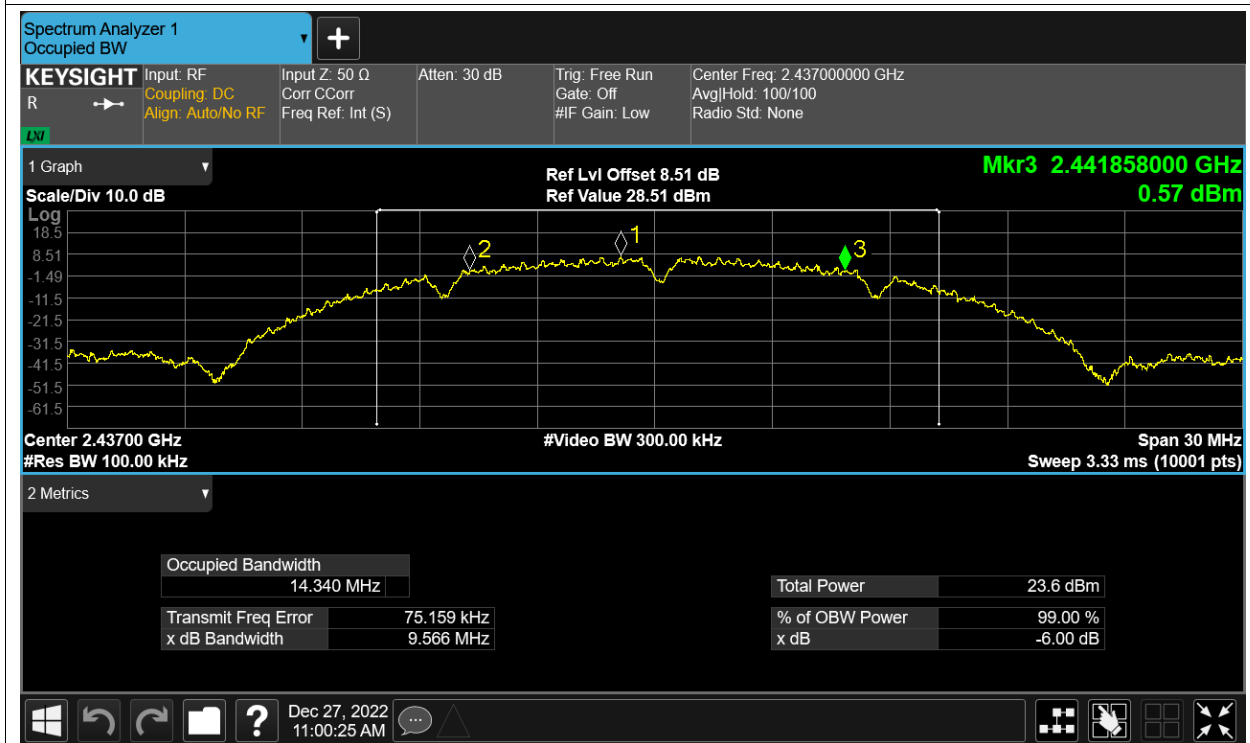
-6dB Bandwidth NVNT b 2462MHz Ant2
