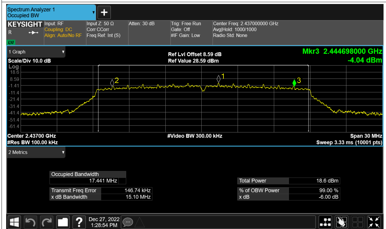
-6dB Bandwidth NVNT n20 2437MHz Ant2
