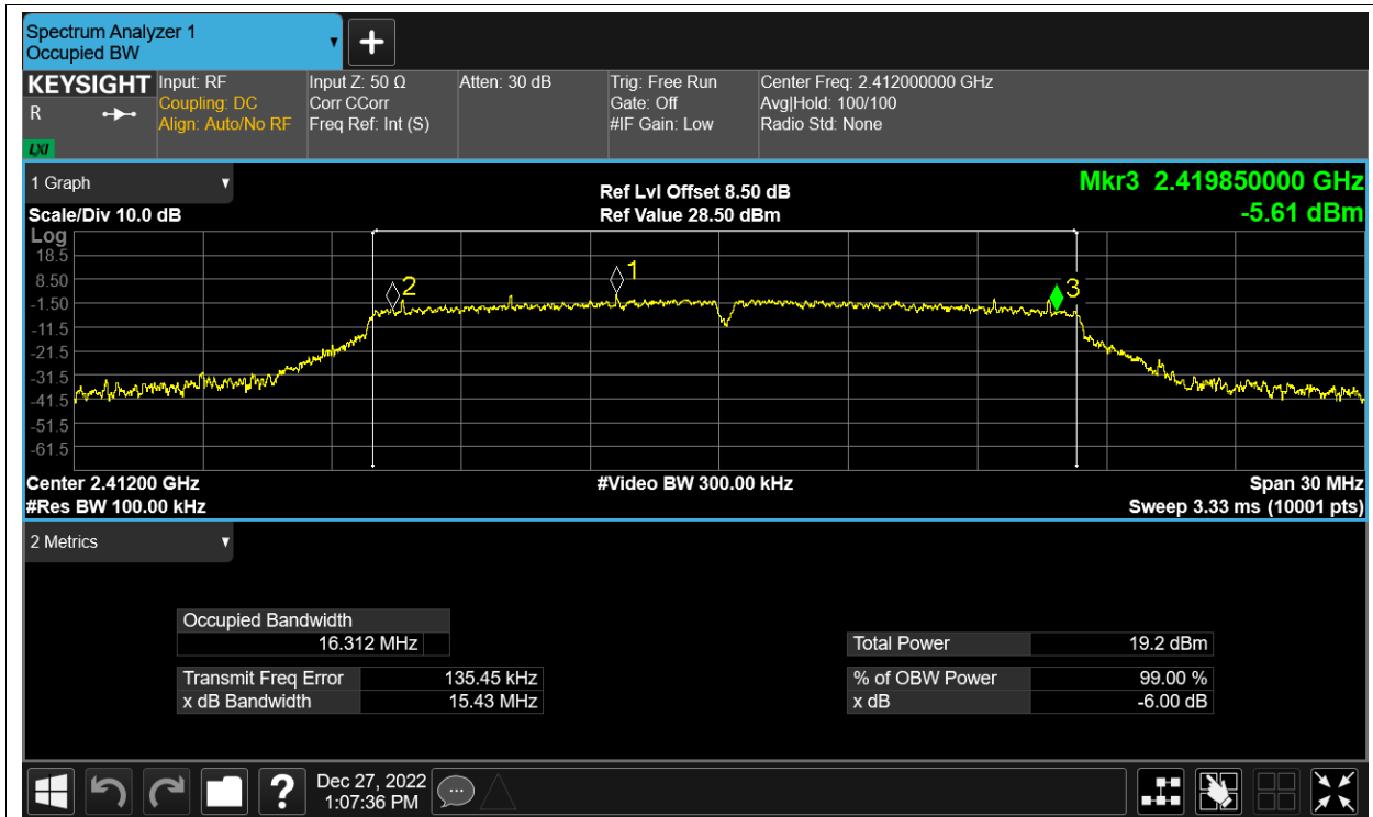
-6dB Bandwidth NVNT g 2437MHz Ant2
