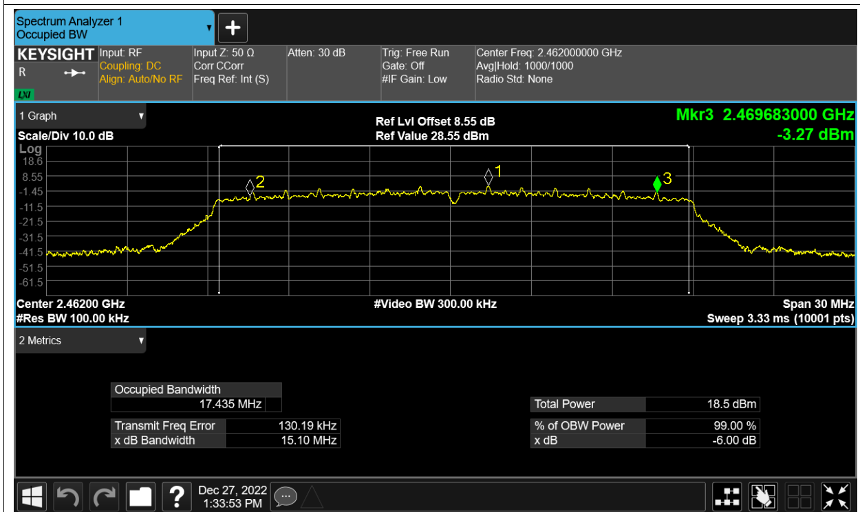
-6dB Bandwidth NVNT n20 2462MHz Ant2
