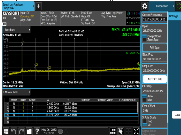
Spurious Emission BLE 1M HighCH39-2480MHz
