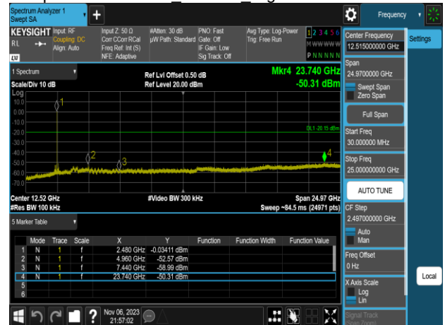
Spurious Emission BLE 2M HighCH39-2480MHz
