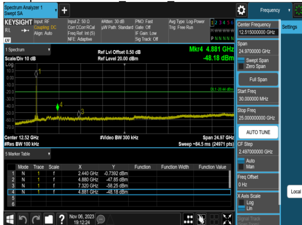
Spurious Emission BLE 1M HighCH39-2480MHz
