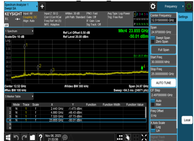
Spurious Emission BLE 2M HighCH39-2480MHz
