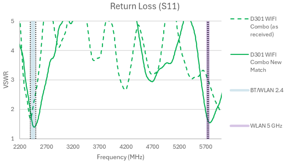
Figure 8 - VSWR Comparison (original vs. updated WIFI COMBO antenna matching)
