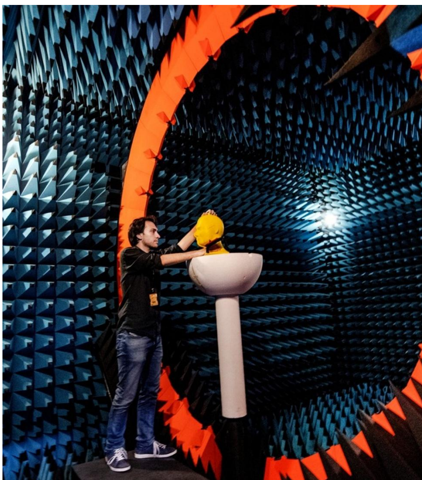
Figure 55 - Satimo Chamber with phantom head
