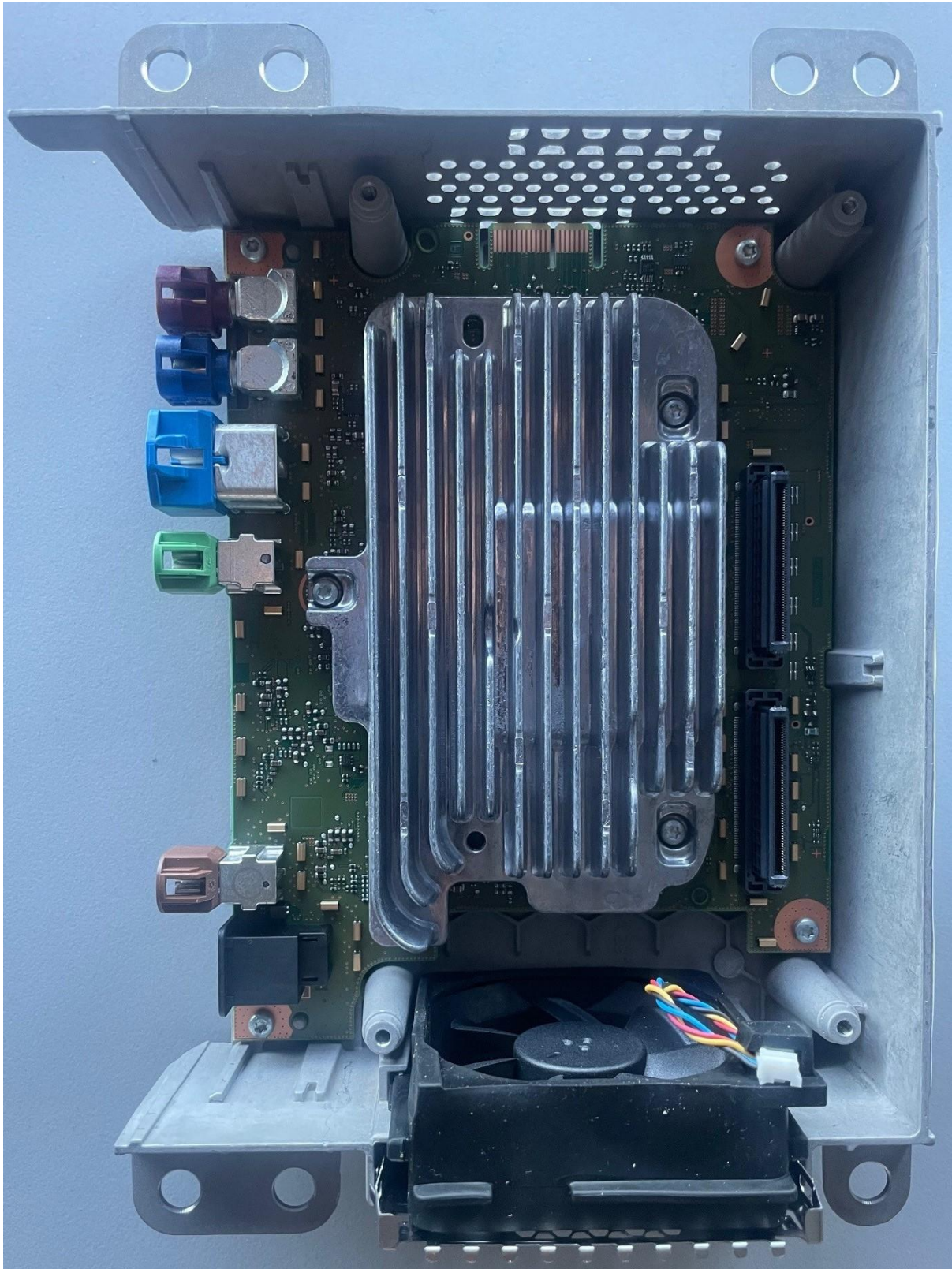
MMB mounted with heatsink
