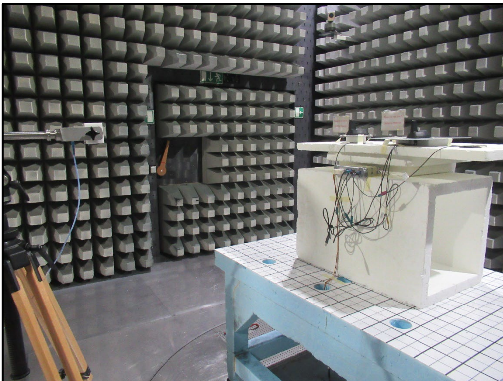
Photo 8 Radiated Test Setup from 18 GHz to 40 GHz
