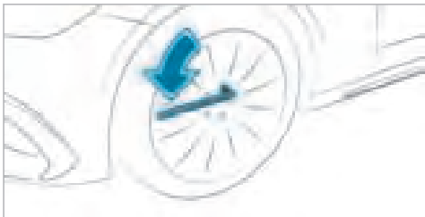
Position of the jack support points
