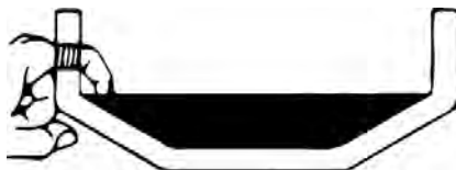
Figure 59: Improper Oil Level
