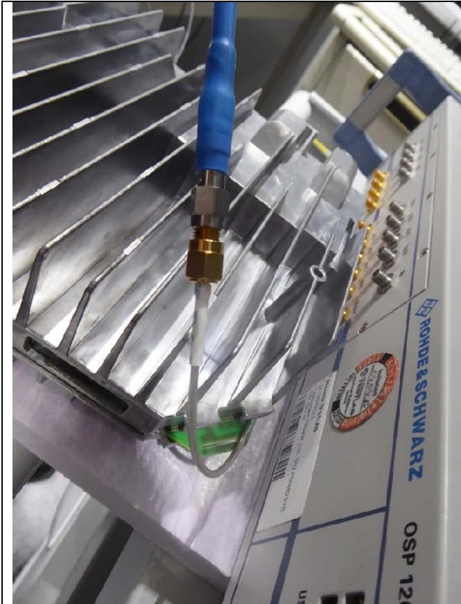
Internal antenna: Temporary antenna connector
