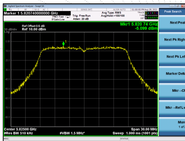
(802.11n20) PSD plot on channel 165
