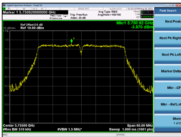
(802.11n40) PSD plot on channel 159
