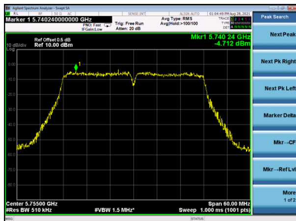
(802.11ac40) PSD plot on channel 159
