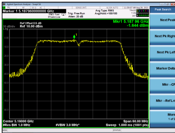
(802.11n40) PSD plot on channel 46
