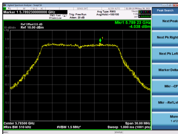
(802.11a) PSD plot on channel 165
