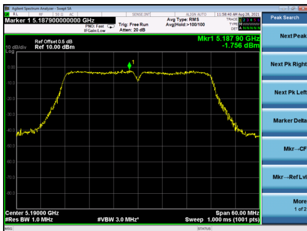
(802.11ac40) PSD plot on channel 46
