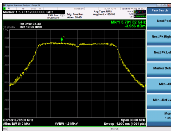
(802.11ac20) PSD plot on channel 165
