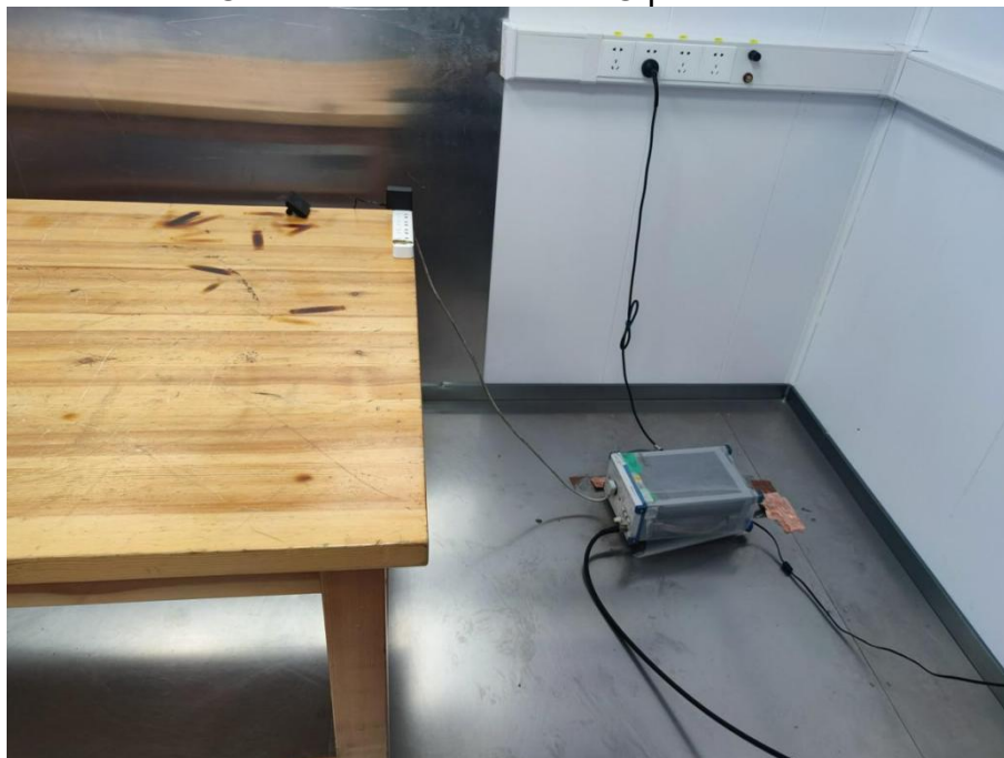
Conducted Emission at AC power line
