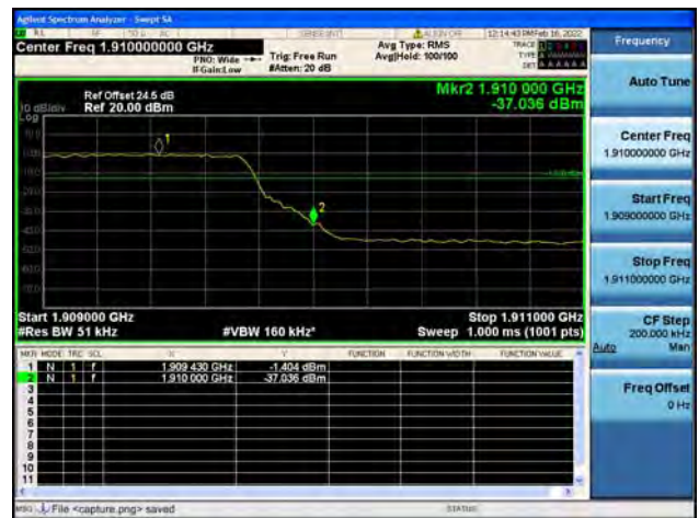
Band2 / 5MHz / High CH / QPSK / FULL RB
