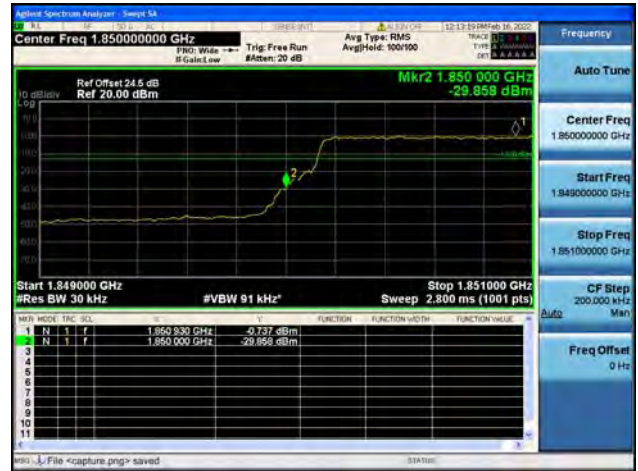
Band2 / 3MHz / High CH / QPSK / FULL RB
