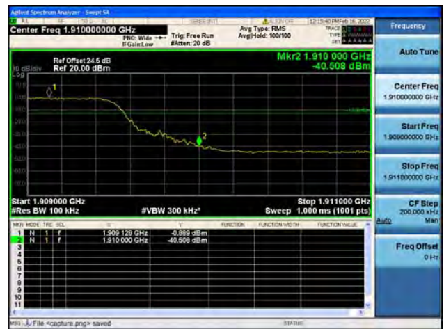
Band2 / 10MHz / High CH / QPSK / FULL RB
