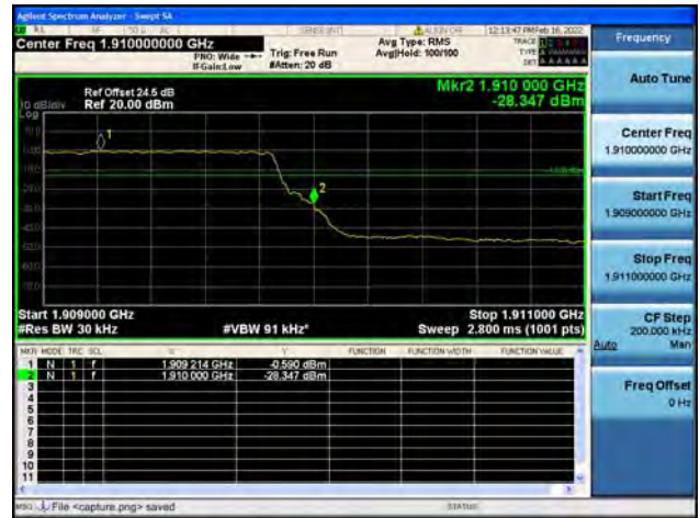
Band2 / 3MHz / High CH / QPSK / FULL RB
