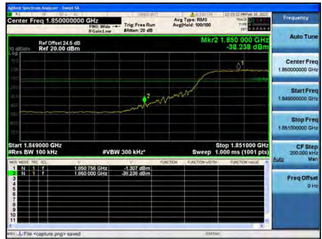
Band2 / 10MHz / High CH / QPSK / FULL RB
