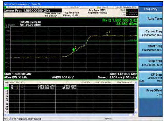
Band2 / 5MHz / High CH / QPSK / FULL RB
