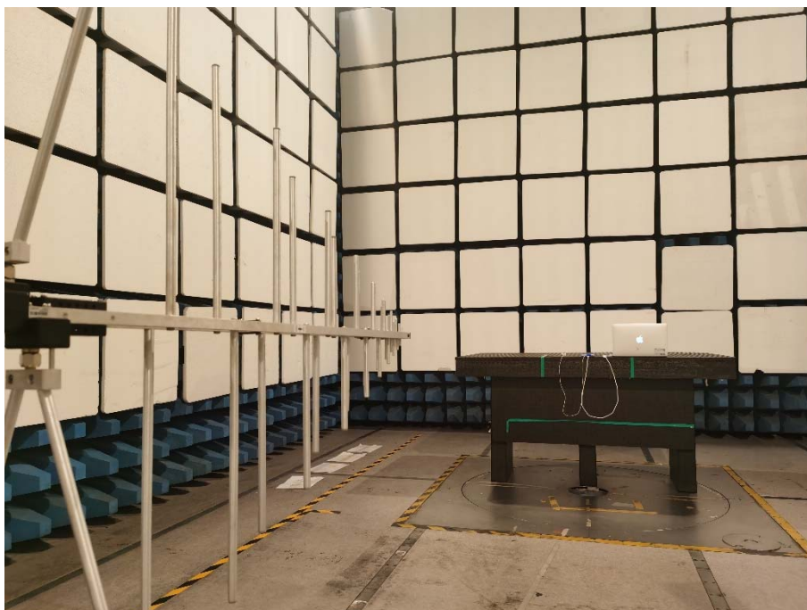
Below 1 GHz, The USB Test Mode
