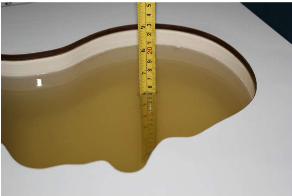
Picture 7-6: Liquid depth in the Head Phantom(2550MHz)
