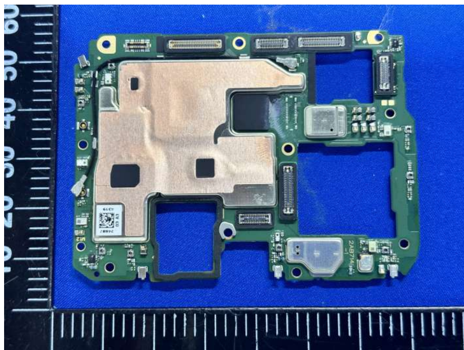
MAIN BOARD TOP VIEW (WITH SHIELDING)
