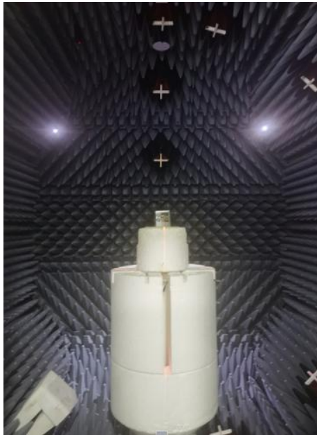
Fig.5. The DUT in the fully anechoic chamber
