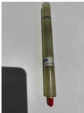
Fig 2 dipole model 3126-2500 frequency 2500 MHz
