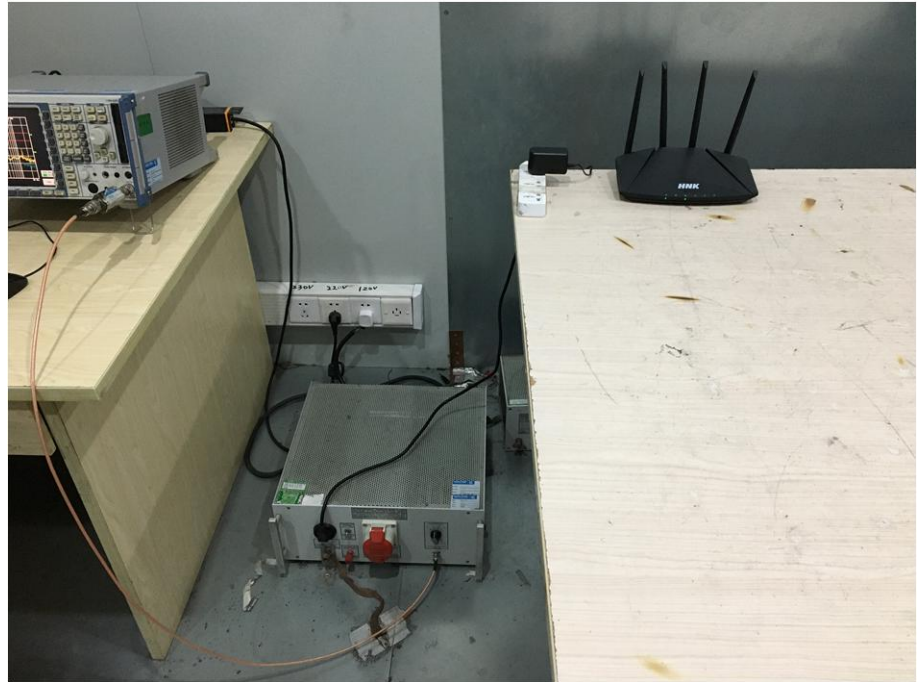
Conducted Emission Test Setup
