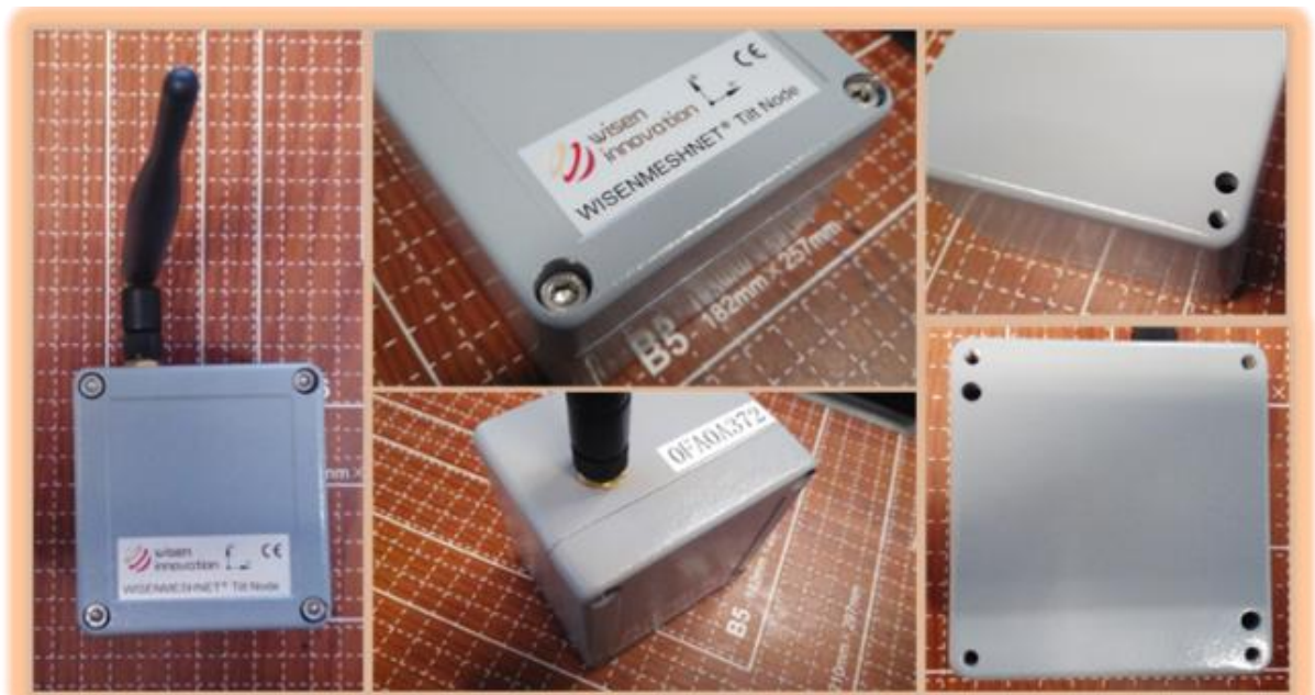
Figure 1. Tilt Node Overview in Photos.
