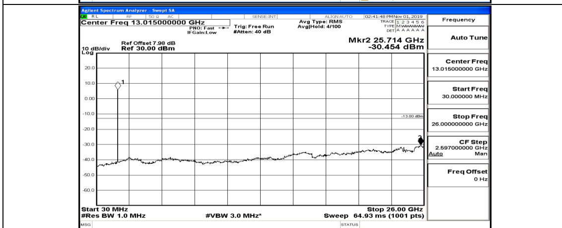
(Channel Bandwidth:15 MHz)_LCH_16QAM_1RB#0
