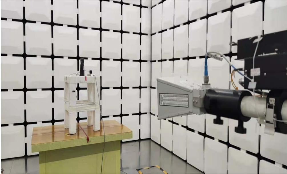
Radiated Spurious Emission Test (1GHz-18GHz)
