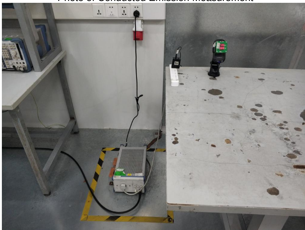
FCC ID: 2AV2W-AH01 Photo of Conducted Emission Measurement
