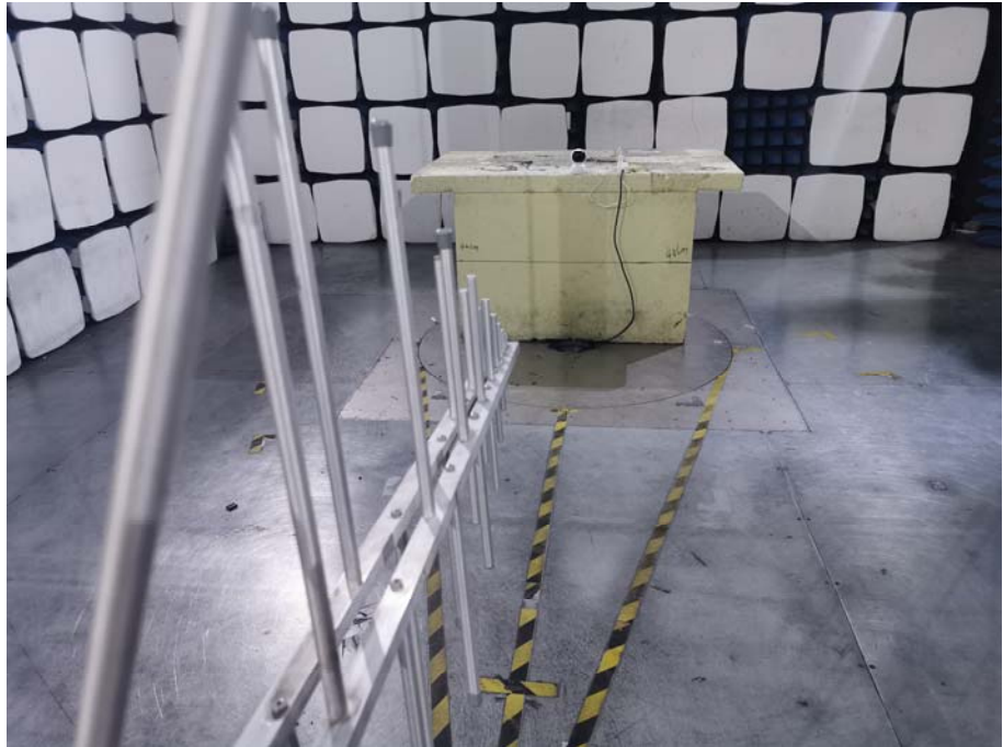
Radiation Emission Test Setup (30MHz to 1GHz)
