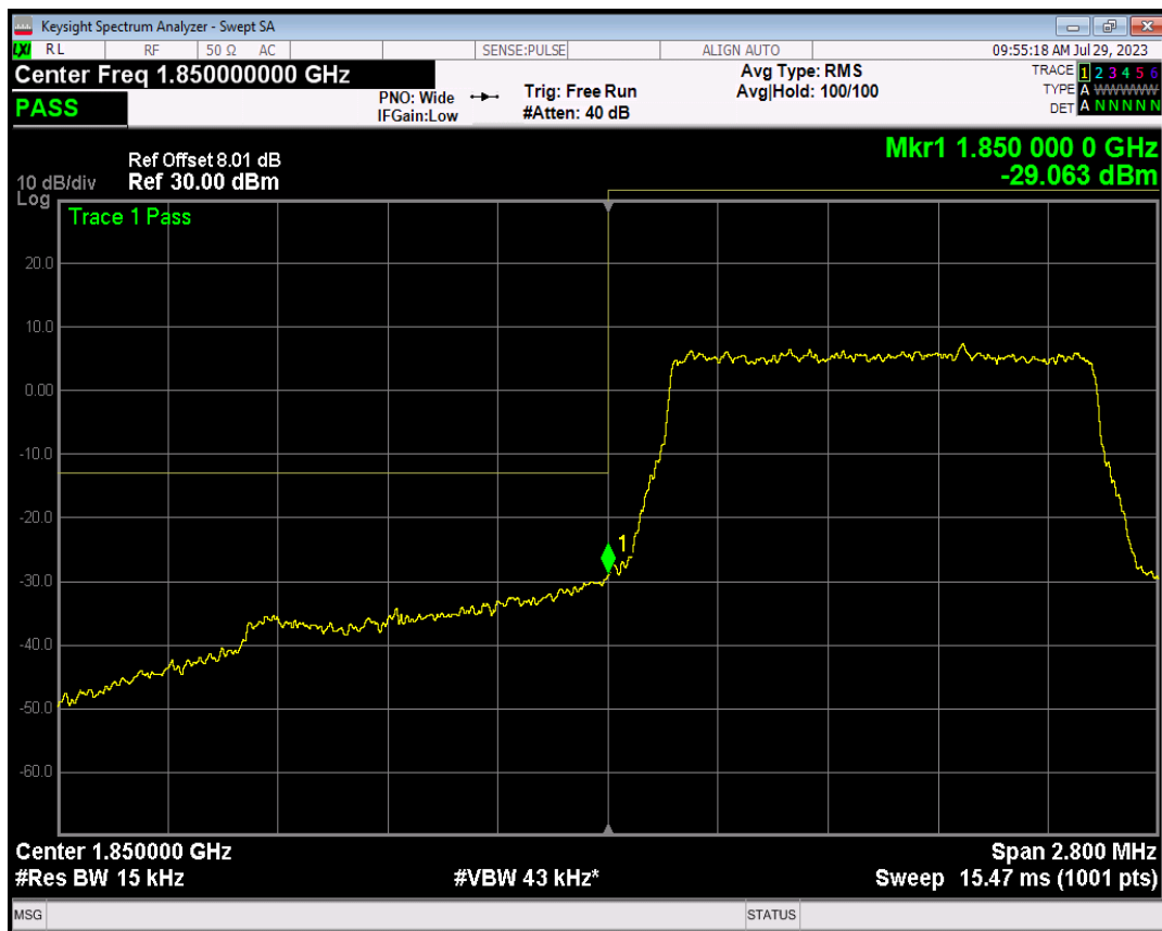
Band2 16QAM BW=1.4MHz Channel=18607 RB Size=1 Position=#0
