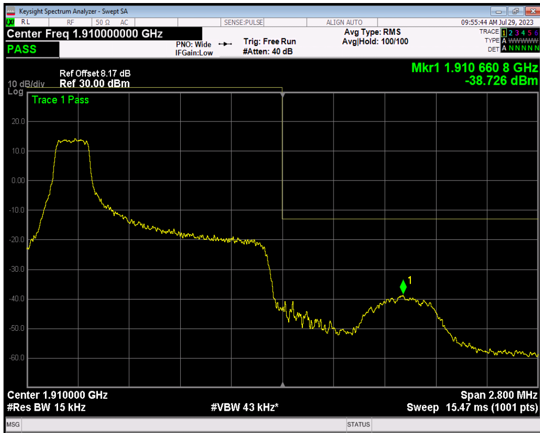
Band2 16QAM BW=1.4MHz Channel=19193 RB Size=1 Position=#Max
