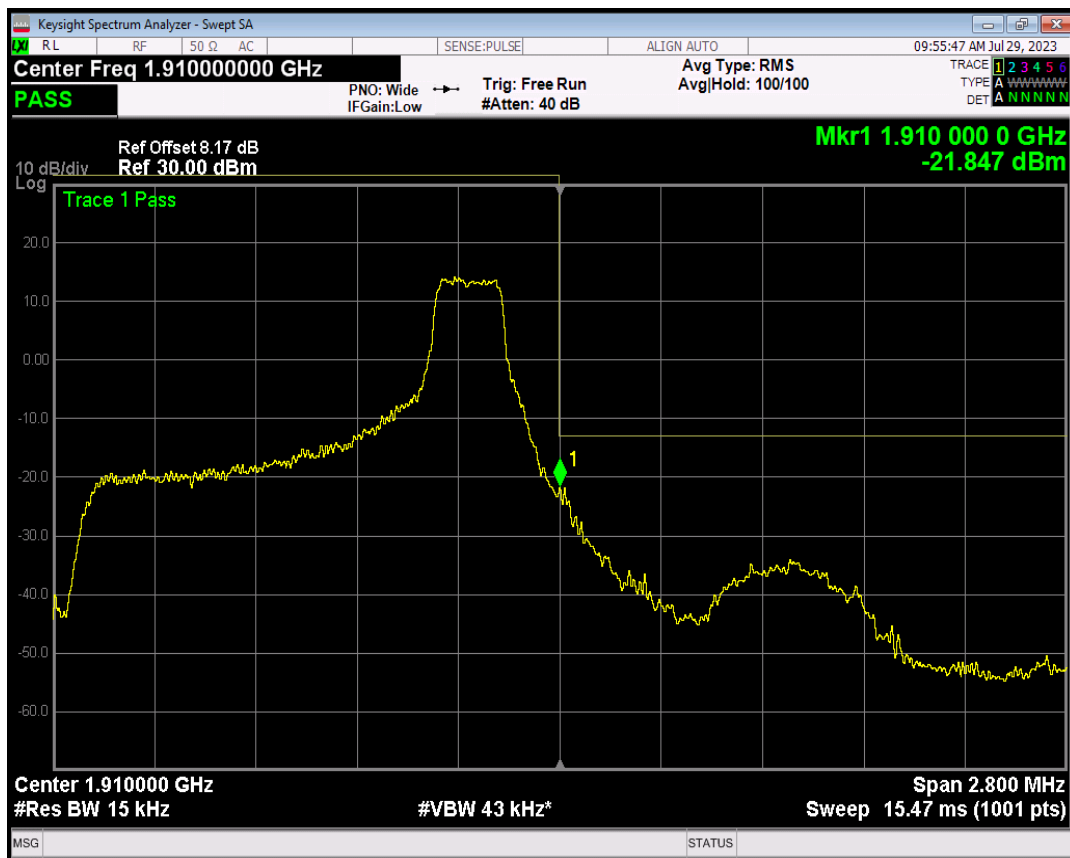
Band2 16QAM BW=1.4MHz Channel=19193 RB Size=6 Position=#0
