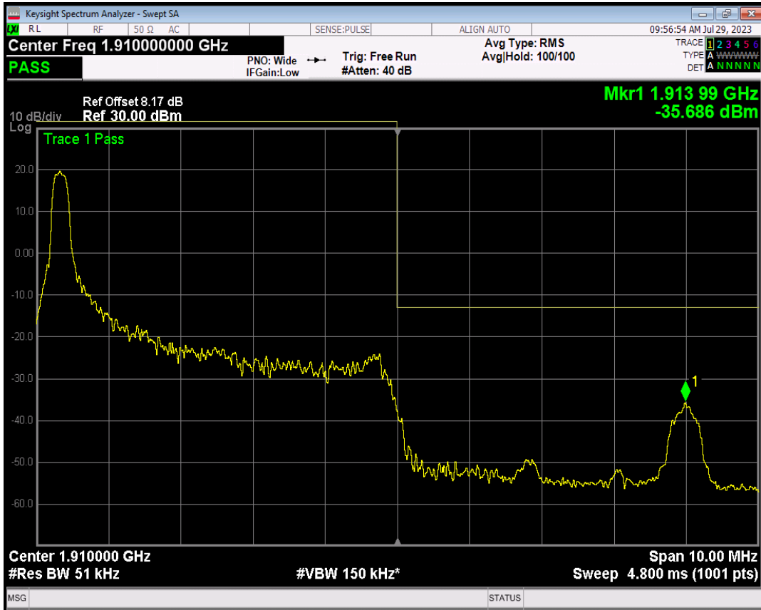
Band2 16QAM BW=5MHz Channel=19175 RB Size=1 Position=#Max
