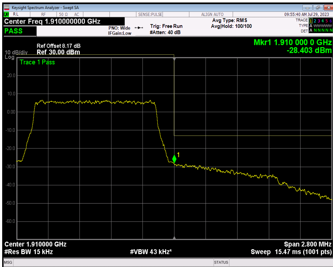
Band2 16QAM BW=1.4MHz Channel=19193 RB Size=1 Position=#0
