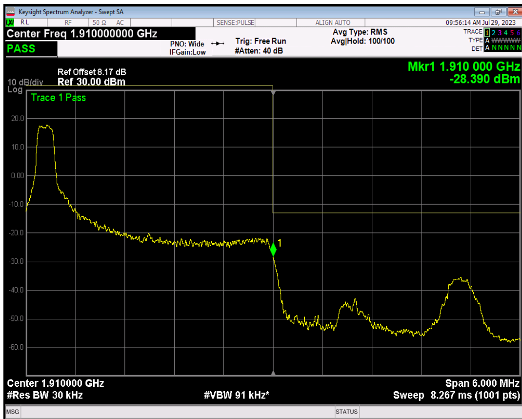
Band2 QPSK BW=3MHz Channel=19185 RB Size=1 Position=#Max
