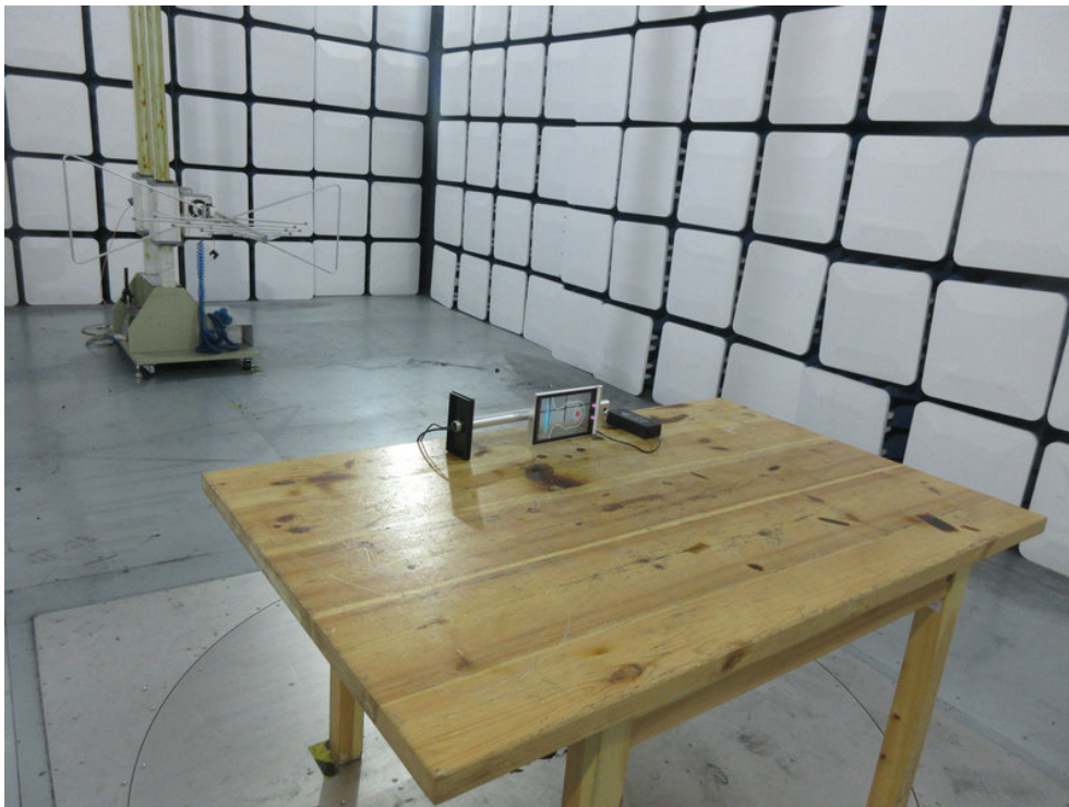
Photo of Radiation Emission Test
