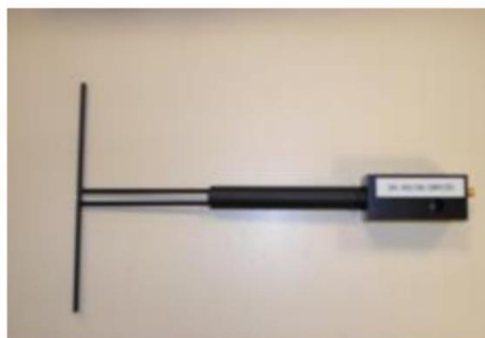
Figure 1 – Satimo COMOSAR Validation Dipole
