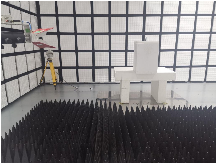
Description: Radiated Emission Test Setup (1 GHz -18GHz)
