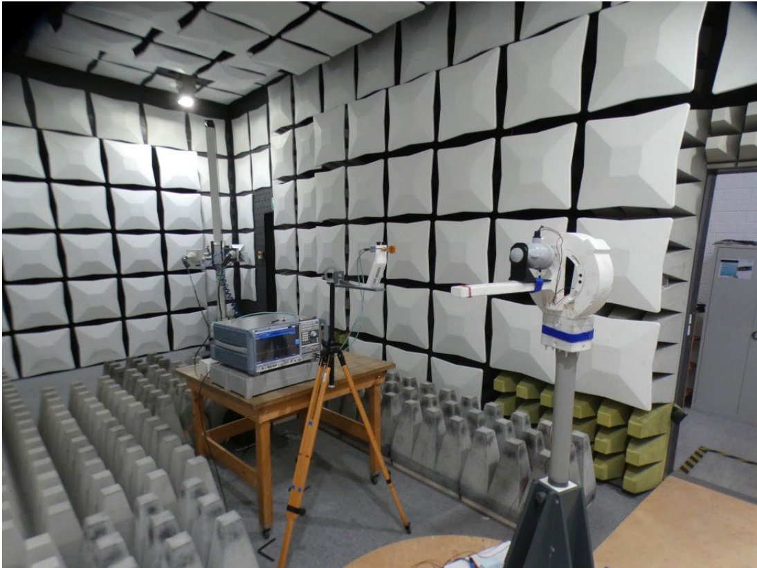
Photo 11: Test setup for radiated antenna pattern measurements 79 GHz (rear side view)
