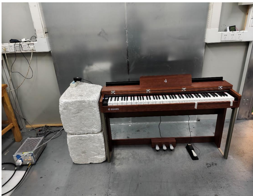
Description: AC Conducted Emissions Test Setup Photo
