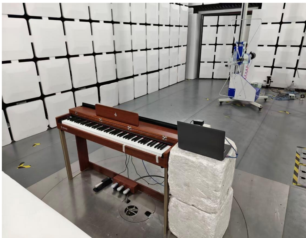
Description: RF Radiated Emission Test Setup for 30MHz ~ 1GHz
