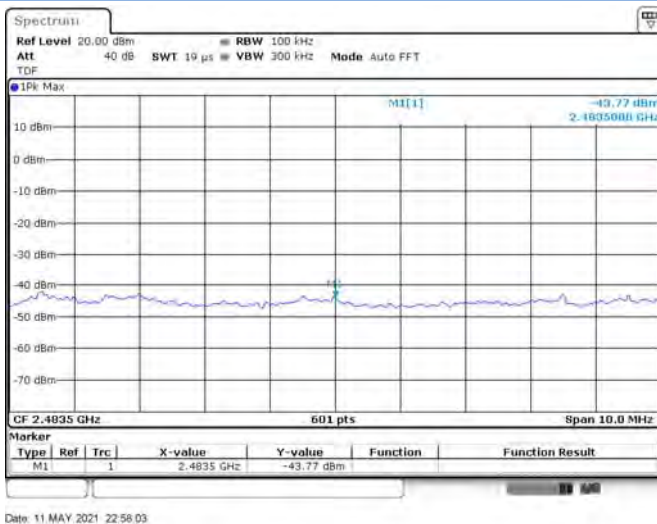
802.11b HIGH CHANNEL, Carrier level
