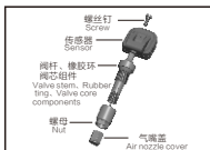
B、内置传感器分解图 Decomposition diagram of built-in sensor
