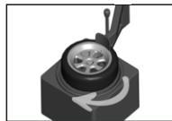
D、从车轮上拆下轮胎 Remove the tire from car wheel
