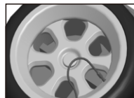
H、将轮胎重新充气 Re-inflating the tires
