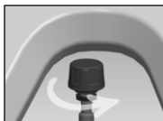
C、用手将防盗六角螺母逆时针方向拧紧,顶着传感器底部 Tighten the nut anticlockwise by hand
