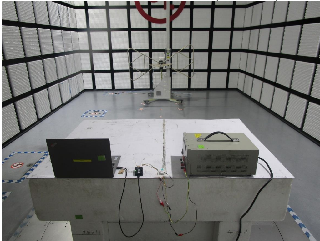
RADIATED RF MEASUREMENT SETUP (Below 30MHz)
