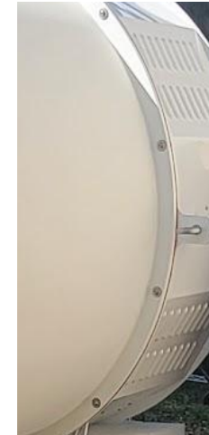
Radome Attachment Bolts (Top Down View)
