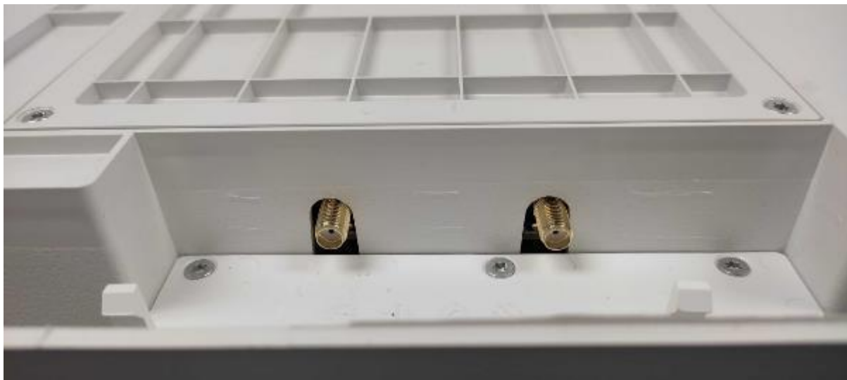
Figure 4: Close up antenna ports at the rear of the cabinet with LTE and Bluetooth antennas removed.
