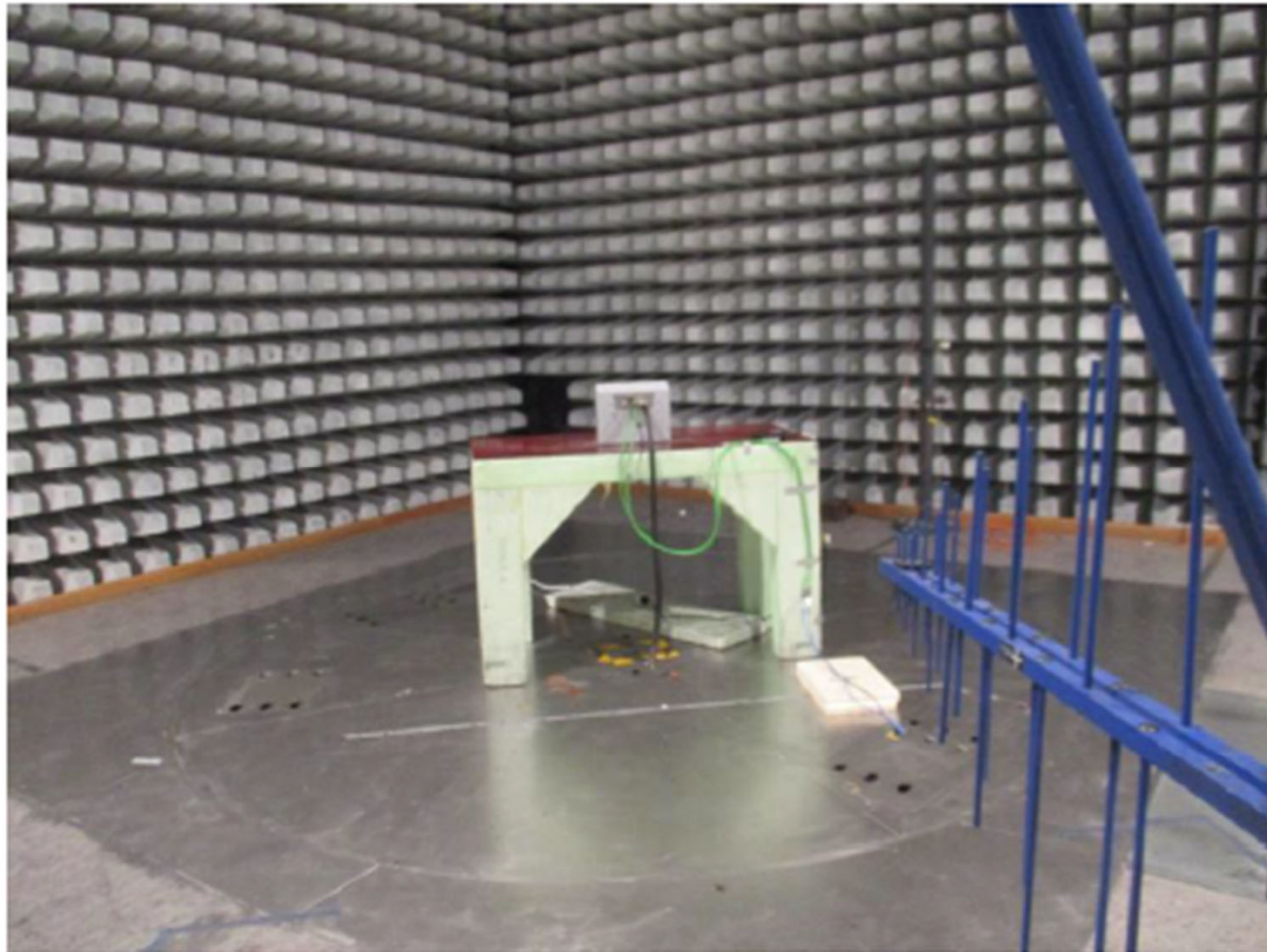
Figure 6-4: test setup for Radiated disturbances 30 MHz to 1000 MHz
