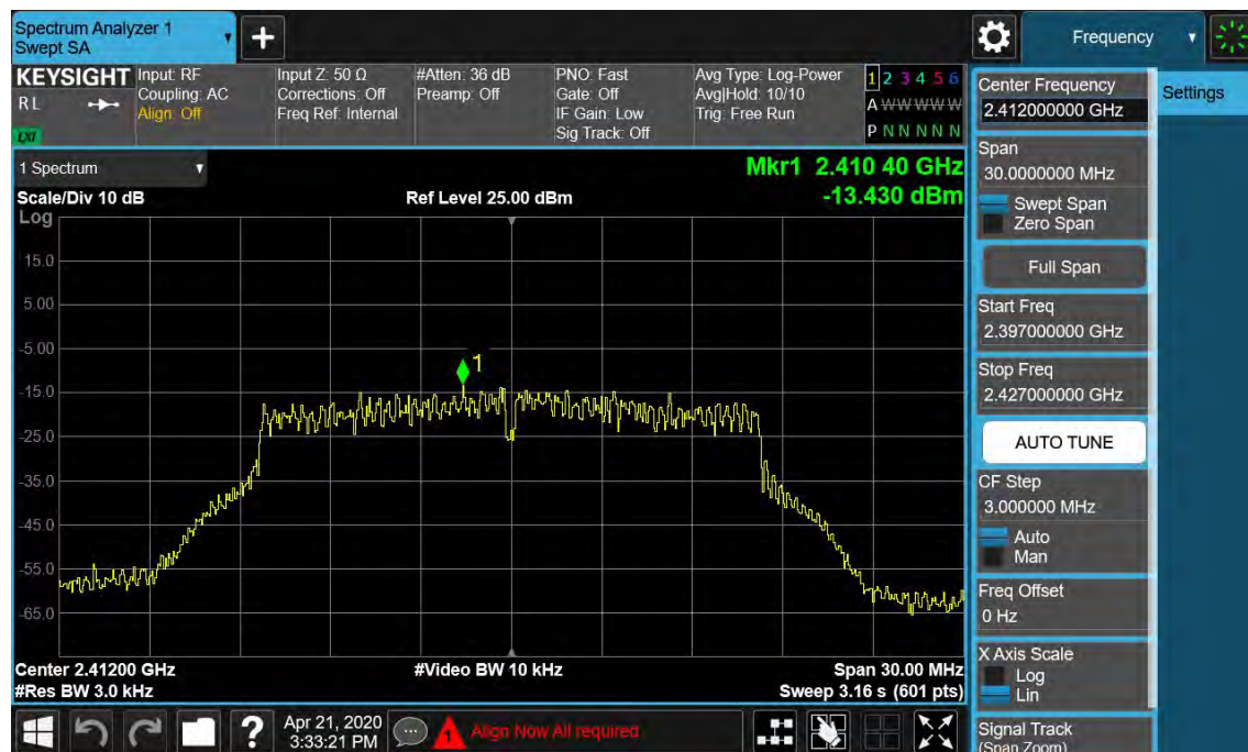
Figure 13: Power Spectral Density, 802.11g, 2412MHz
