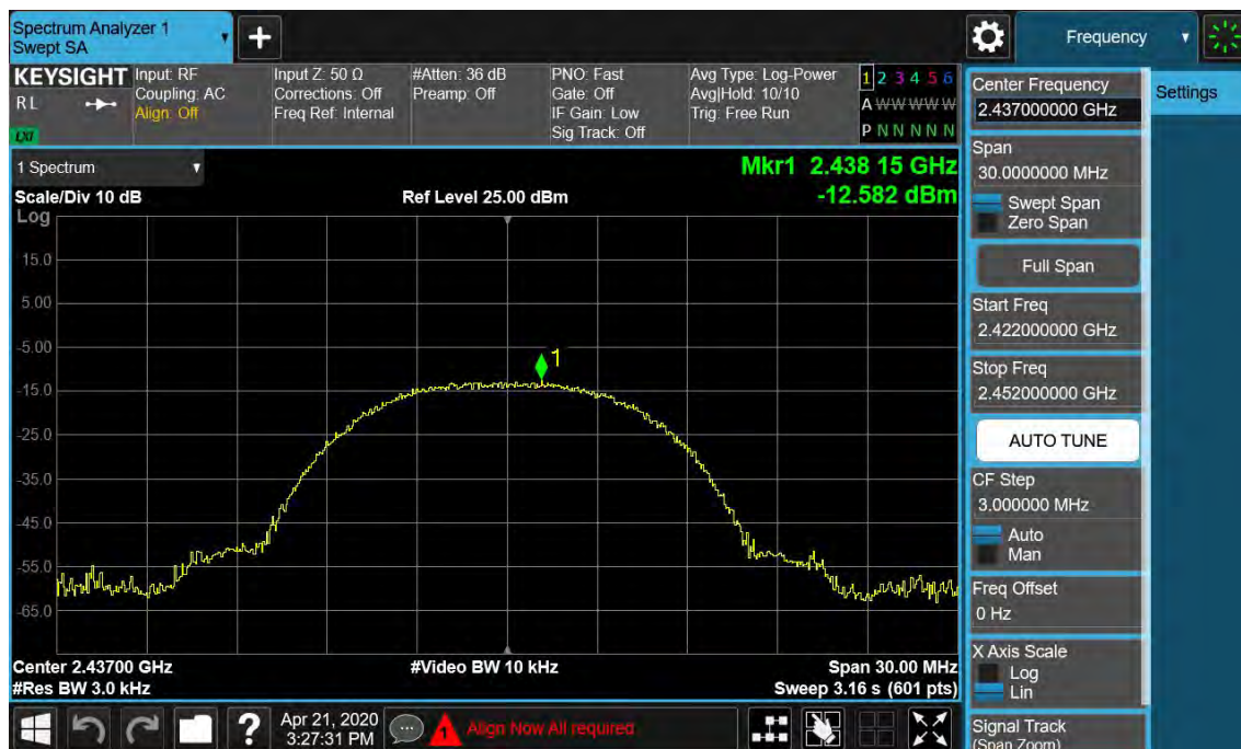
Figure 11: Power Spectral Density, 802.11b, 2437MHz
