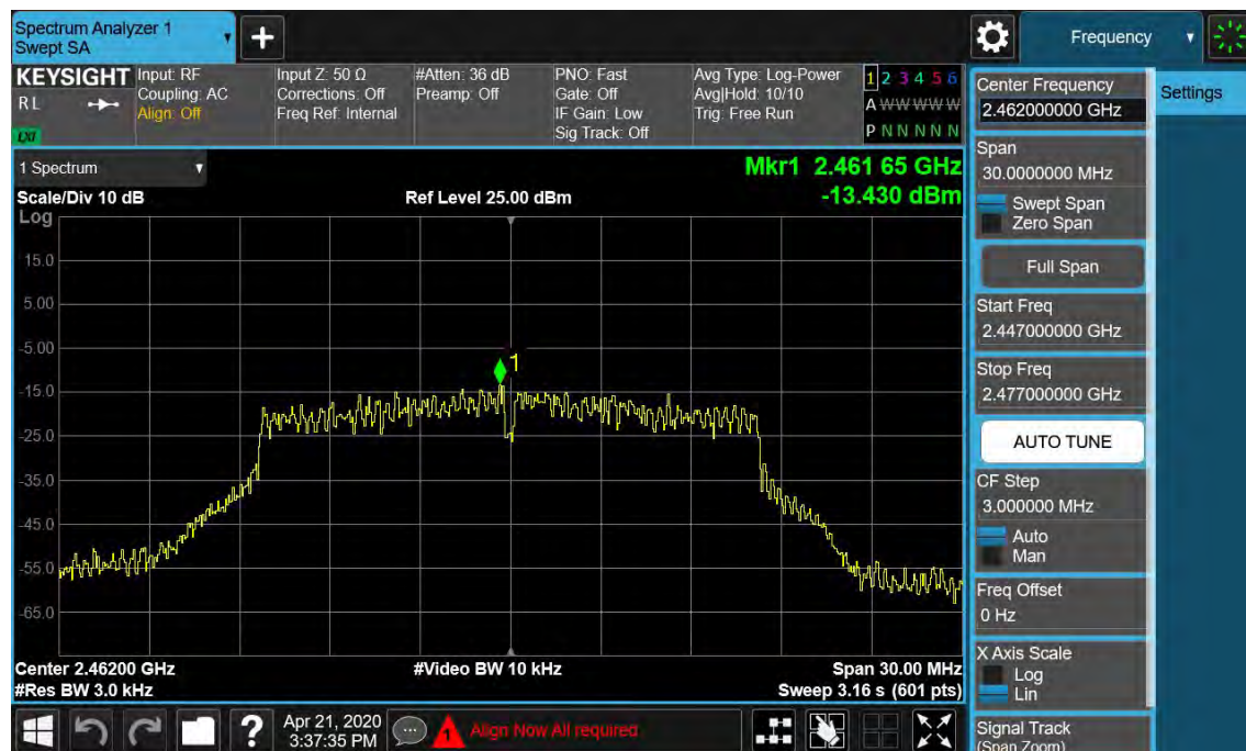
Figure 15: Power Spectral Density, 802.11g, 2462MHz
