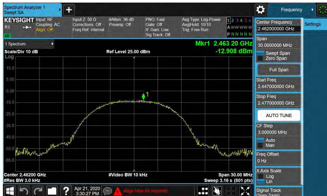
Figure 12: Power Spectral Density, 802.11b, 2462MHz
