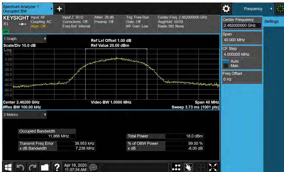
Figure 4: 6dB Bandwidth and 99% Bandwidth, 802.11g, 2412MHz
