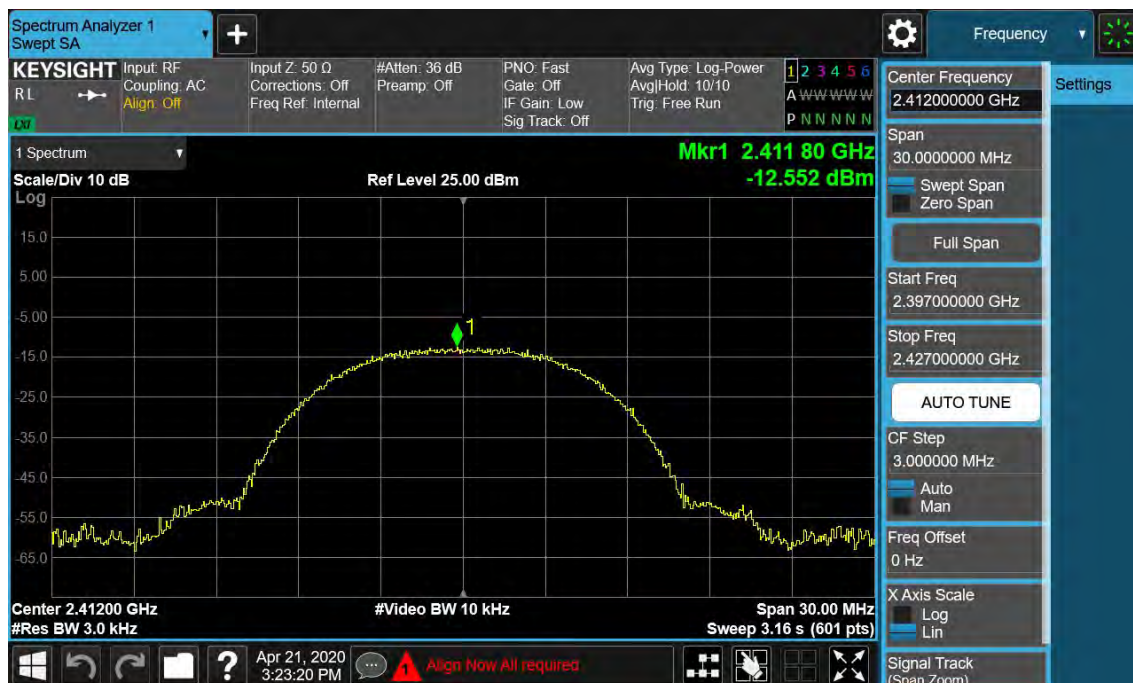
Figure 10: Power Spectral Density, 802.11b, 2412MHz
