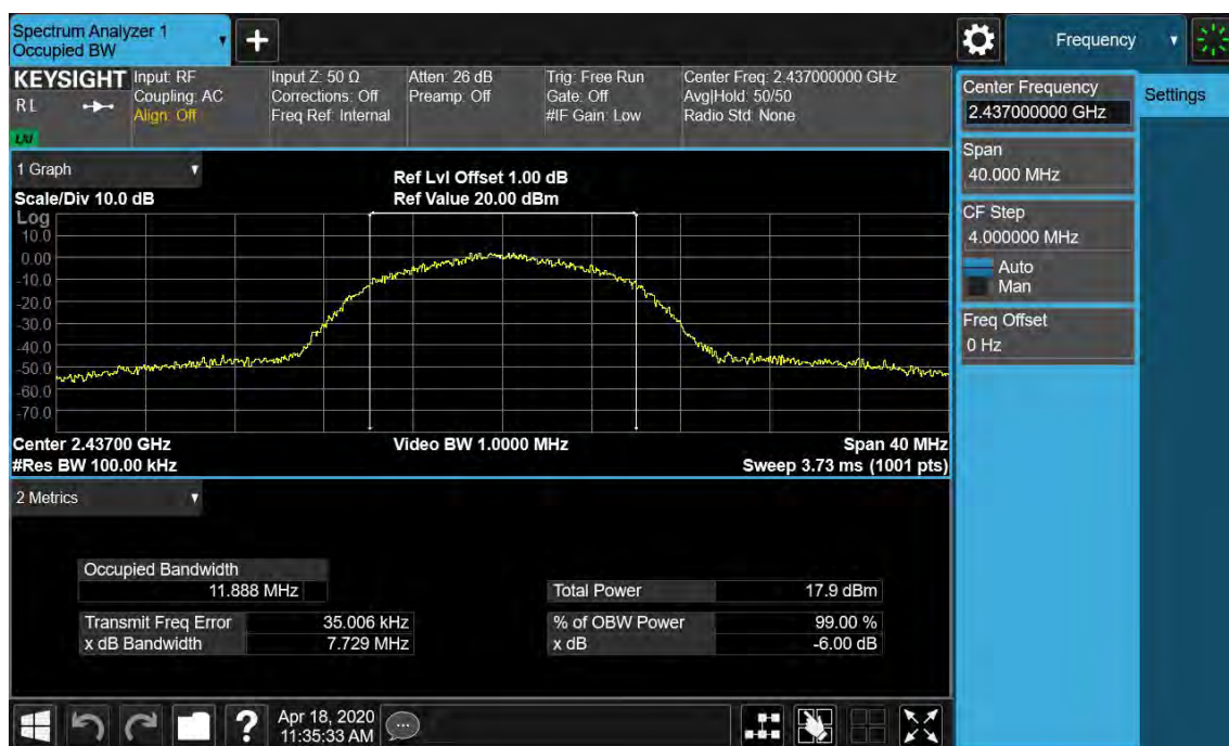
Figure 2: 6dB Bandwidth and 99% Bandwidth, 802.11b, 2437MHz
